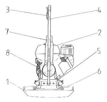
The compact design base plate (1) with centrally mounted, fully enclosed, exciter for an even spread of compactive impact over the whole base plate.
